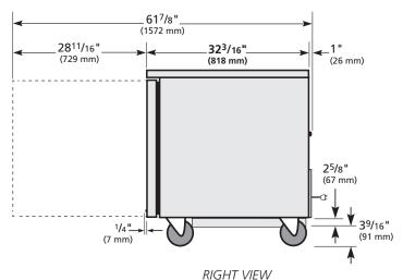
METRIC DIMENSIONS ROUNDED UP TO THE NEAREST WHOLE MILLIMETER
