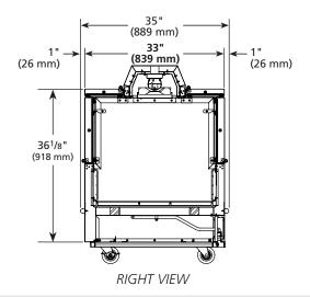
METRIC DIMENSIONS ROUNDED UP TO THE NEAREST WHOLE MILLIMETER
