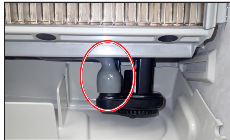
Fig. 9. Disconnect the line from the circulation pump.
