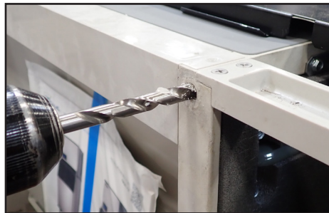
Fig. 3. Drill out the existing hole.
