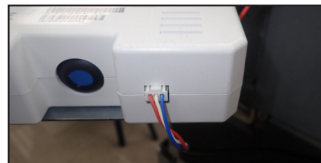
Fig. 5. Blue, Red, & White wire harness connected to the TrueZone.
