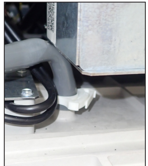
Fig. 13. Tightened snap hose clamp.
