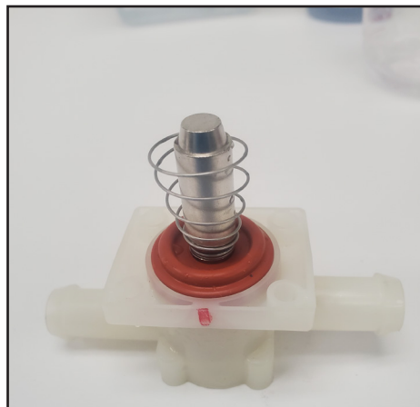
Fig. 3. Rinse all descaler off the valve body and plunger assembly.
