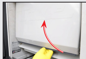
Fig. 2. Push down the damper and pull the water curtain's bottom forward.
