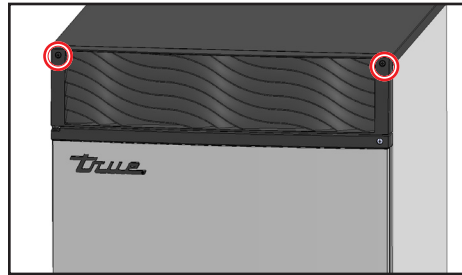
Fig. 4. TCIM-622/822: Front filter grill screw locations.
