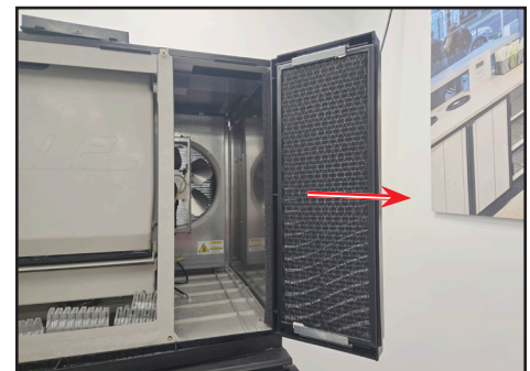
Fig. 2. Slide the air filter out of the brackets.
