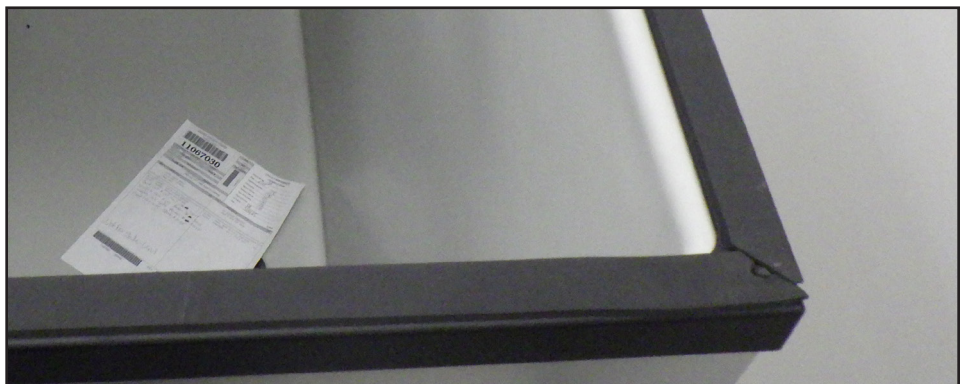
Fig. 2. Reattach the gasket tape to the bin.
