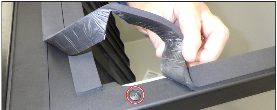
Fig. 1. Carefully lift the gasket tape in the bin corners. Remove the existing screws.
