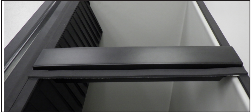
Fig. 1. Measure and center the bin adapter on the bin.
