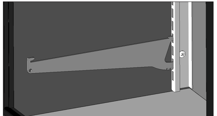
Fig. 14. Installed shelf support bracket.
