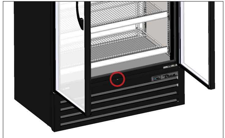
Fig. 2. Front louver grill screw location.
