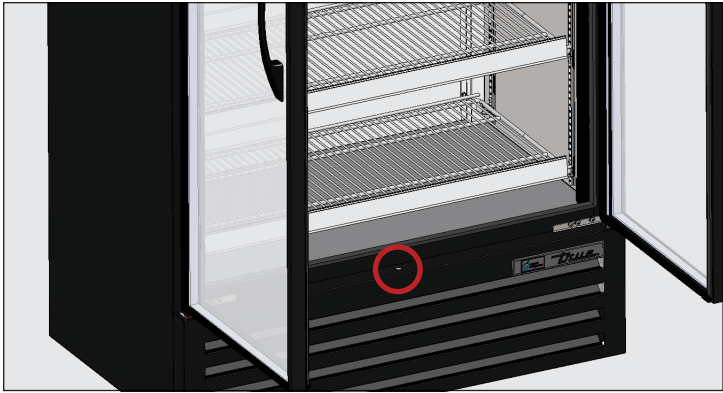
Fig. 1. Swing door louver grill screw location.
