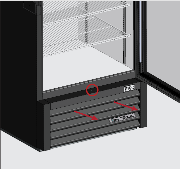
Fig. 3. Front louver grill screw location. Carefully remove the grill from the magnets.
