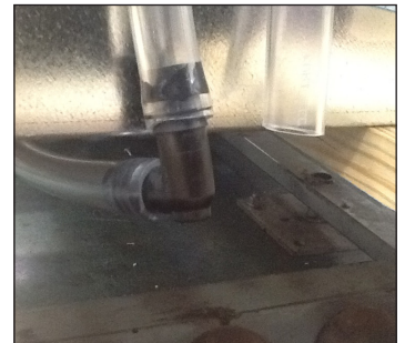
Fig. 6. Connect the barbed fitting to the hoses on the cabinet.
