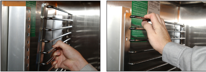
Fig. 7b. Installing kit #2 rod tray sides.
