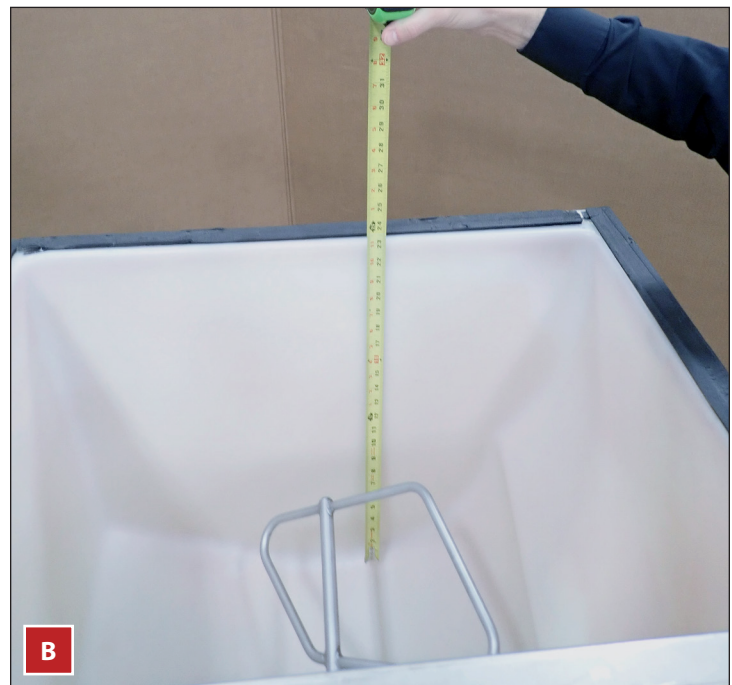
Fig. 2. Always measure the bin (A) or dispenser (B) for the TOF sensor before positioning the TCIM.
