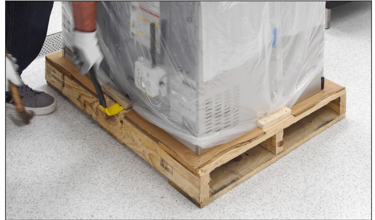
Fig. 1. Remove the wood blocks from the skid.
