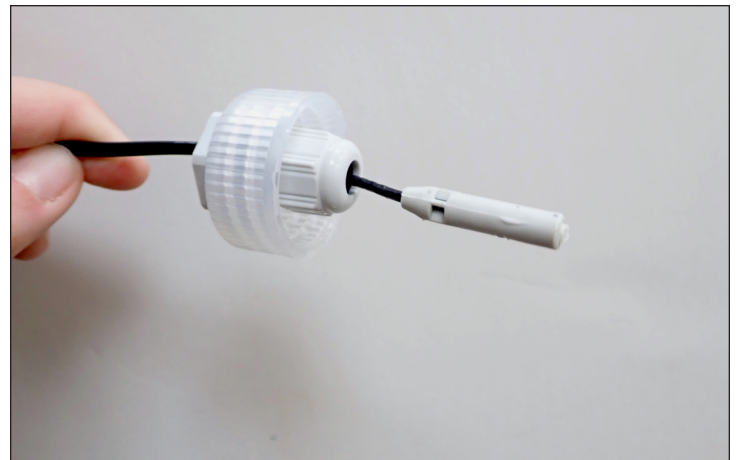
Fig. 2. Black temperature probe through the cap with a hole.
