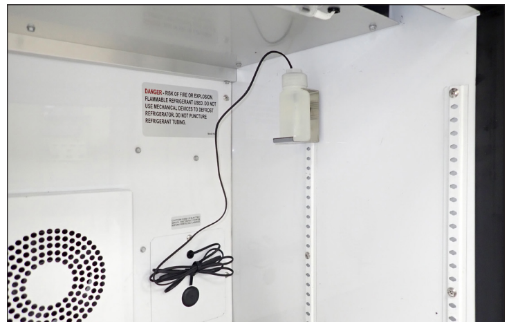
Fig. 4. Undercounter; TRUE recommends installing the glycol bottle assembly at the top of the right rear shelf standard as shown. Glycol bottle bracket installed with an existing shelf standard screw.
