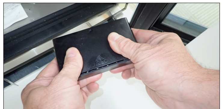
Fig. 8. Slide the battery cover off.
