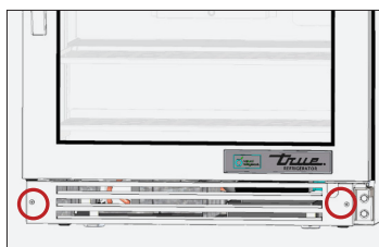
Fig. 6. Undercounter front louver grill screw locations. Grill is magnetically held on once screws are removed.
