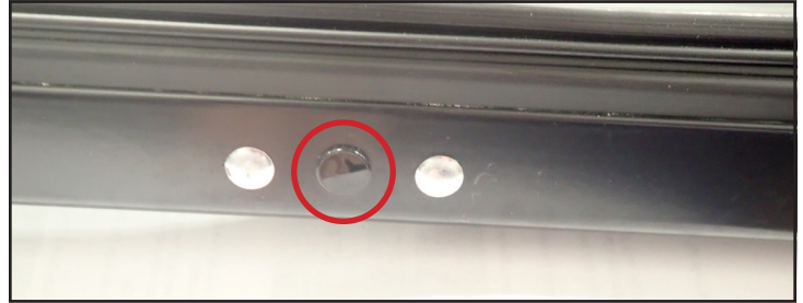
Fig. 22. Plastic cap in the door's bottom.
