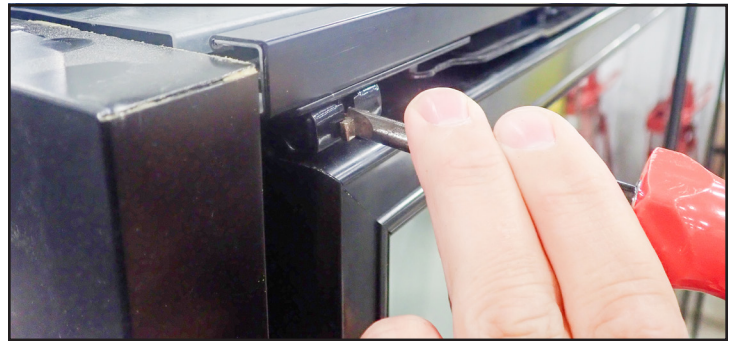
Fig. 14. Open the hinge retention clip.
