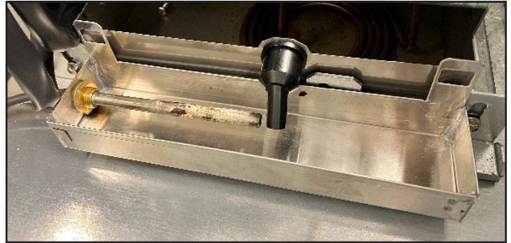
Fig. 2. Position the HDP under the overflow nozzle.
