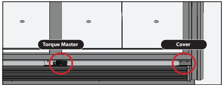
Fig. 25. Original torque master assembly and cover locations.
