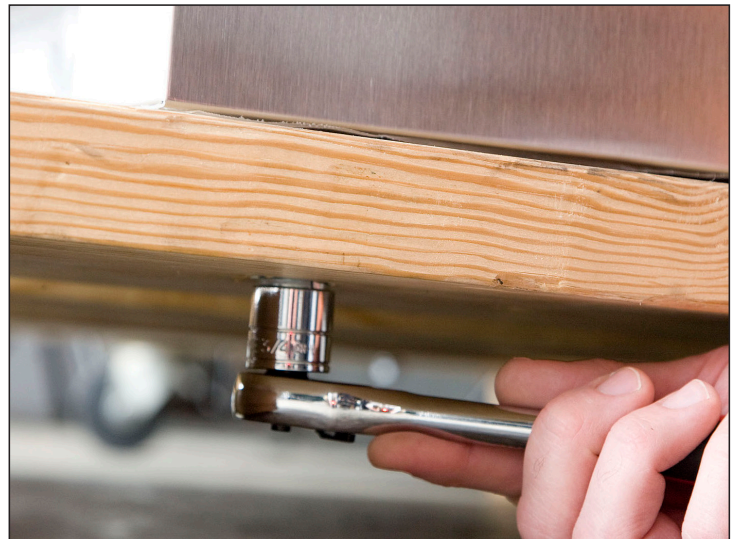
Fig. 3. Remove the skid bolts.
