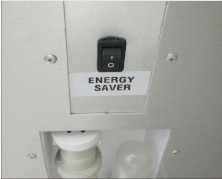
Fig. 1. Energy saver switch.
