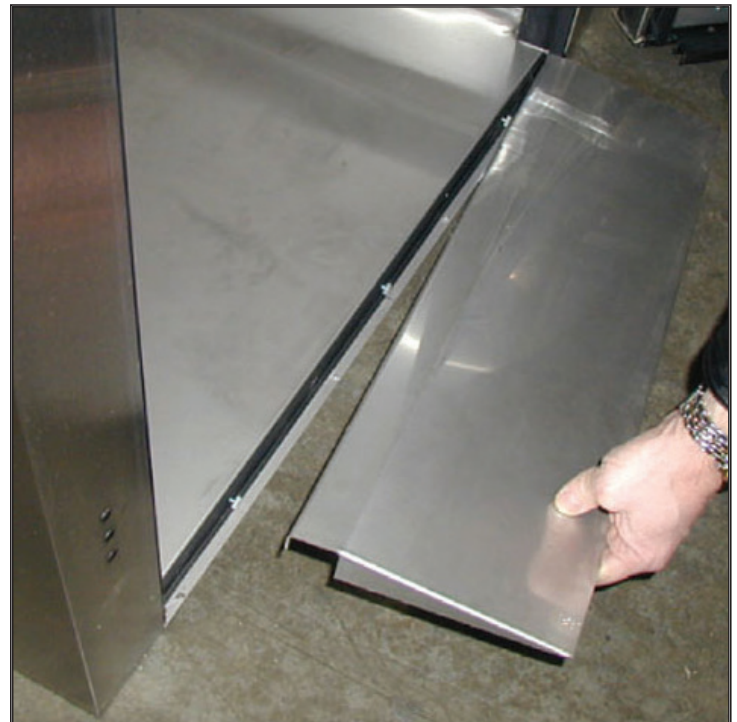
Fig. 2. Slide the ramp onto the thumbscrews.
