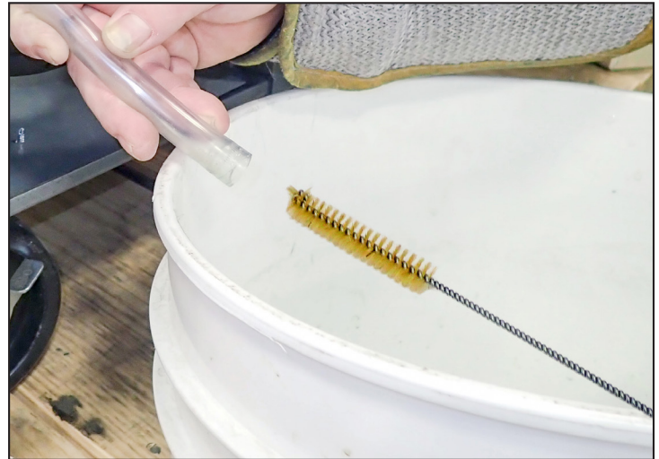
Fig. 2. Catch trapped liquid in a large container.
