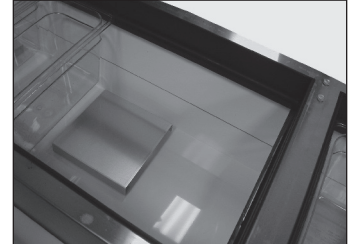
Fig. 2. Correctly positioned baffle.
