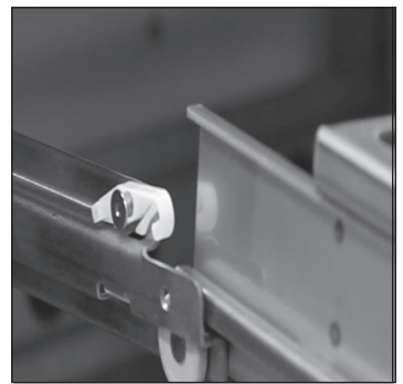
Fig. 7. Align the drawer with the drawer slide.
