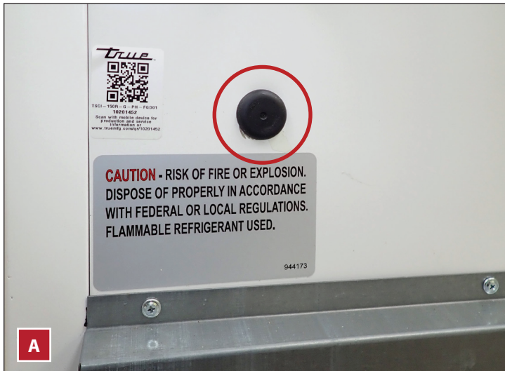
Fig. 2. Undercounter probe port exterior (A) and interior (B) view.
