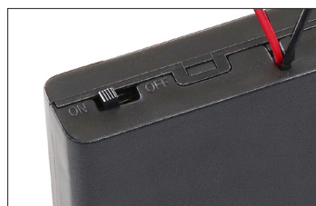
Fig. 7. Battery backup toggled to ON.
