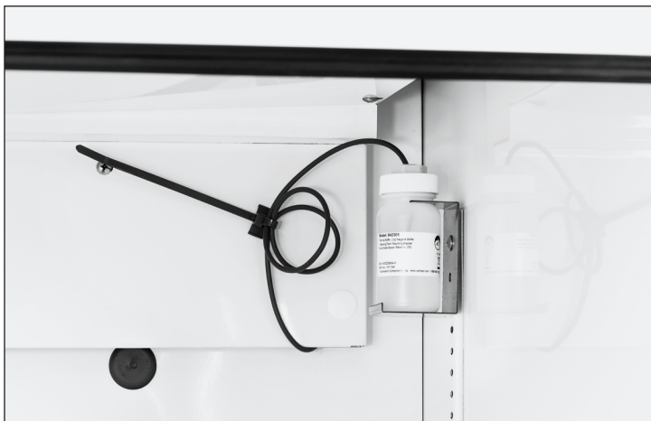
Fig. 3. Upright; TRUE recommends installing the glycol bottle assembly at the top of the right rear shelf standard as shown. Glycol bottle bracket installed with an existing shelf standard screw.
