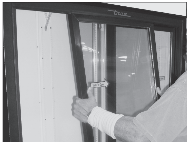
Fig. 3 Carefully remove the door.
