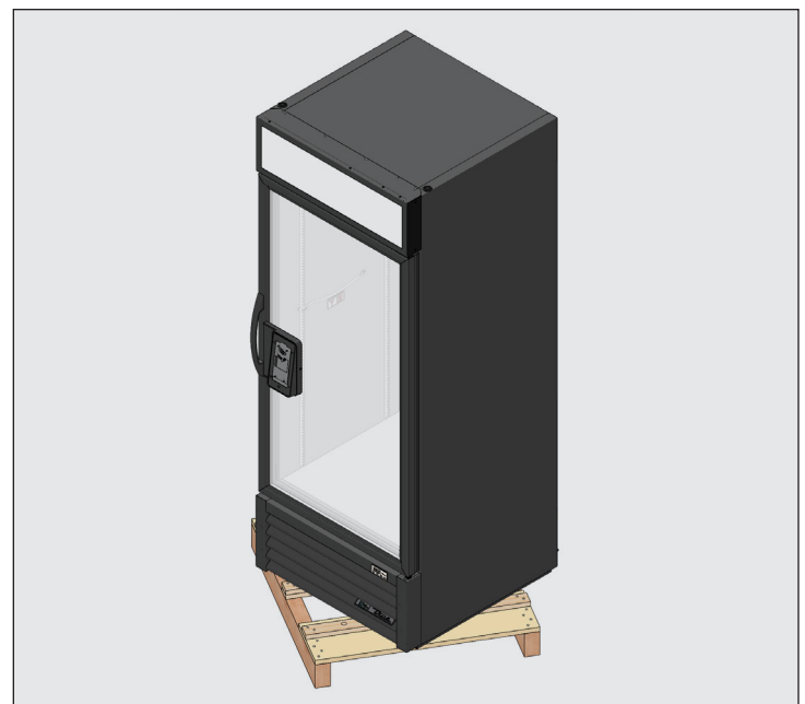
Fig. 4. When lifting appliance, do not use countertops, doors/drawers, or grills as a lifting point.
