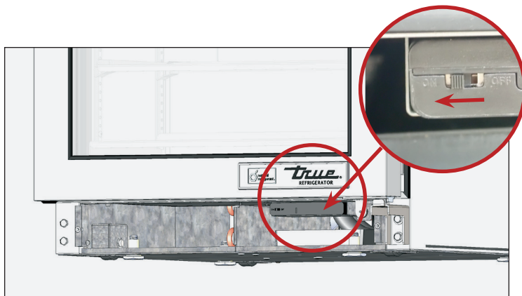
Fig. 4. Undercounter battery backup location.
