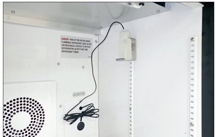
Fig. 4. TRUE recommends installing the glycol bottle assembly at the top of the right rear shelf standard as shown. Glycol bottle bracket installed with an existing shelf standard screw. Undercounter.
