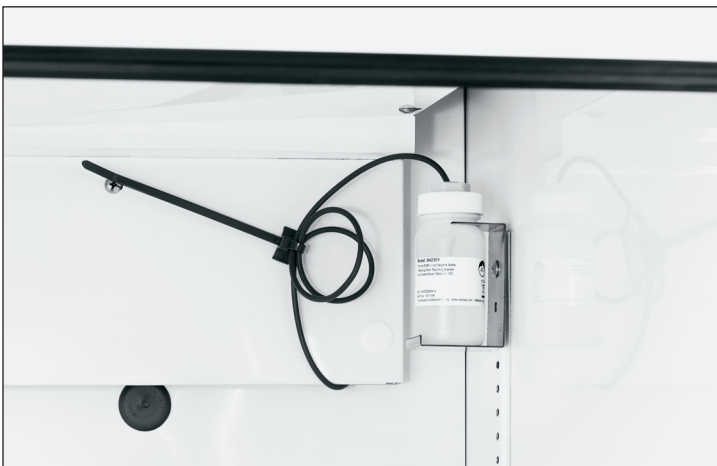
Fig. 3. TRUE recommends installing the glycol bottle assembly at the top of the right rear shelf standard as shown. Glycol bottle bracket installed with an existing shelf standard screw. Upright.
