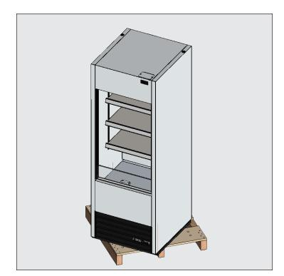
Fig. 3. When lifting the appliance, do not use countertops, doors/drawers, or grills as a lifting point.
