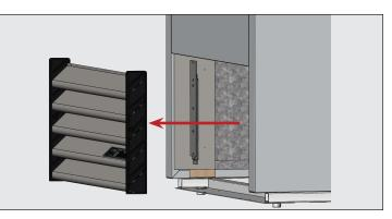
Fig. 2. Pull to remove the lourve grill.
