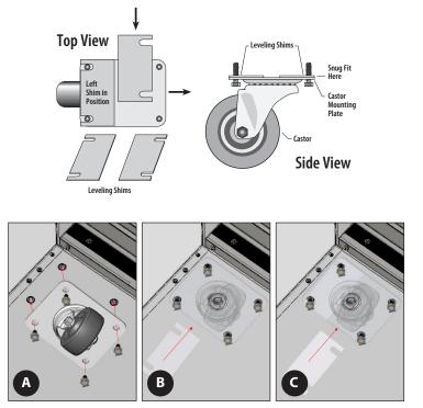
Fig. 7. Install castor shims in pairs.
