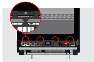
Fig. 3. Remove the front grill bolts to access the shipping bolts.
