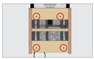
Fig. 2. Example of shipping bolt locations.
