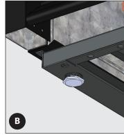
Fig. 2. Turn the leveling screws clockwise to lower the unit.
