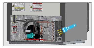
Fig. 4. Verify all blockages have been removed.
