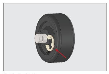
Fig. 13. Install retaining ring.
