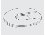
**Fig. 10.** Install multiple shims with offset slots.
