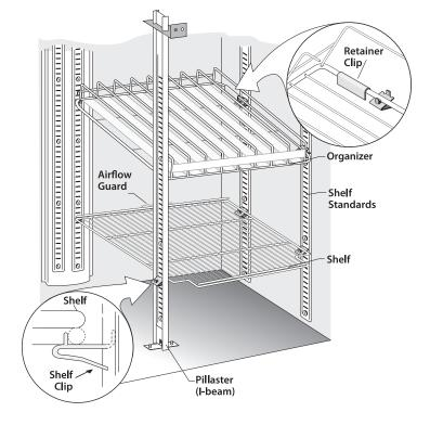
Fig. 5. Installed shelf clip.
