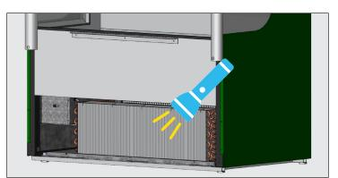
Fig. 5. Verify all blockages have been removed.
