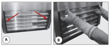
Fig. 1. Louver grill screw location (A). Pull the grill from the appliance front (B).
