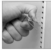
Fig. 6. Installing top tab of shelf clip.
