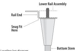
Fig. 4. Leveling leg diagram.
