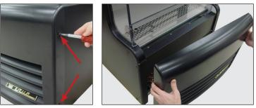
Fig. 2. TAC-14GS-HC-LD Grill removal. Lift grill away from cabinet after removing screws.
