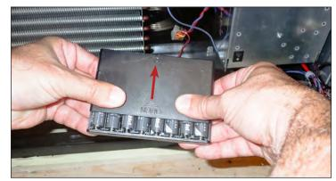
Fig. 4. Slide the battery cover off.
