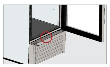
Fig. 1. Remove the top screw from the louver grill.
