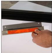
Fig. 2. Remove the glass swing door shipping bracket. Do not discard.
