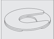
**Fig. 10.** Install multiple shims with offset slots.
