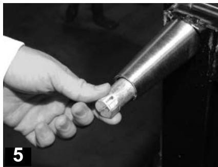
5 The end of the leg is adjustable to easy leveling.
