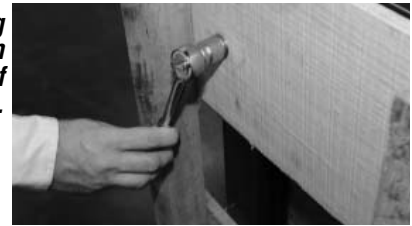
Removing skid from bottom of cabinet.
